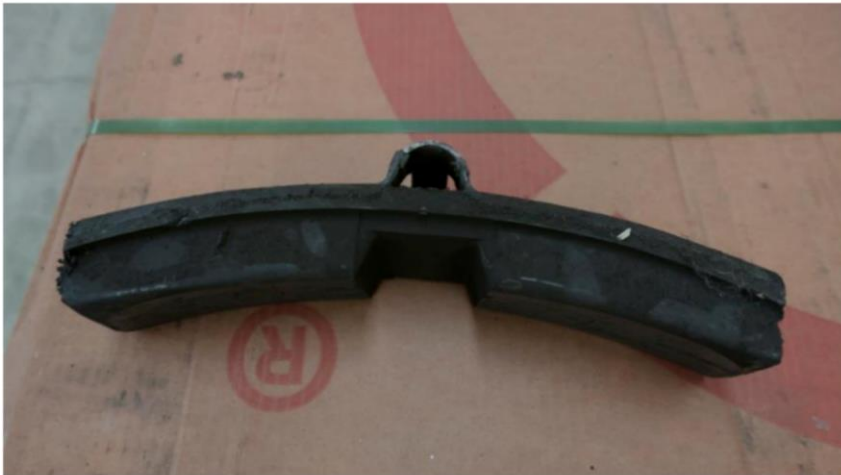
A new unworn brake for the locomotive
